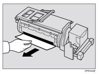
**3** Remove paper that is stuck to the drum.
